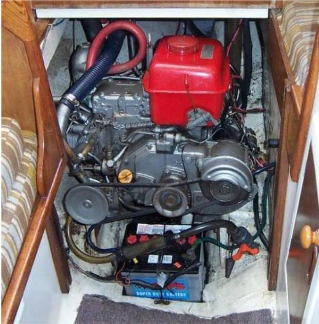
**Diesel motor in Compass 28**
