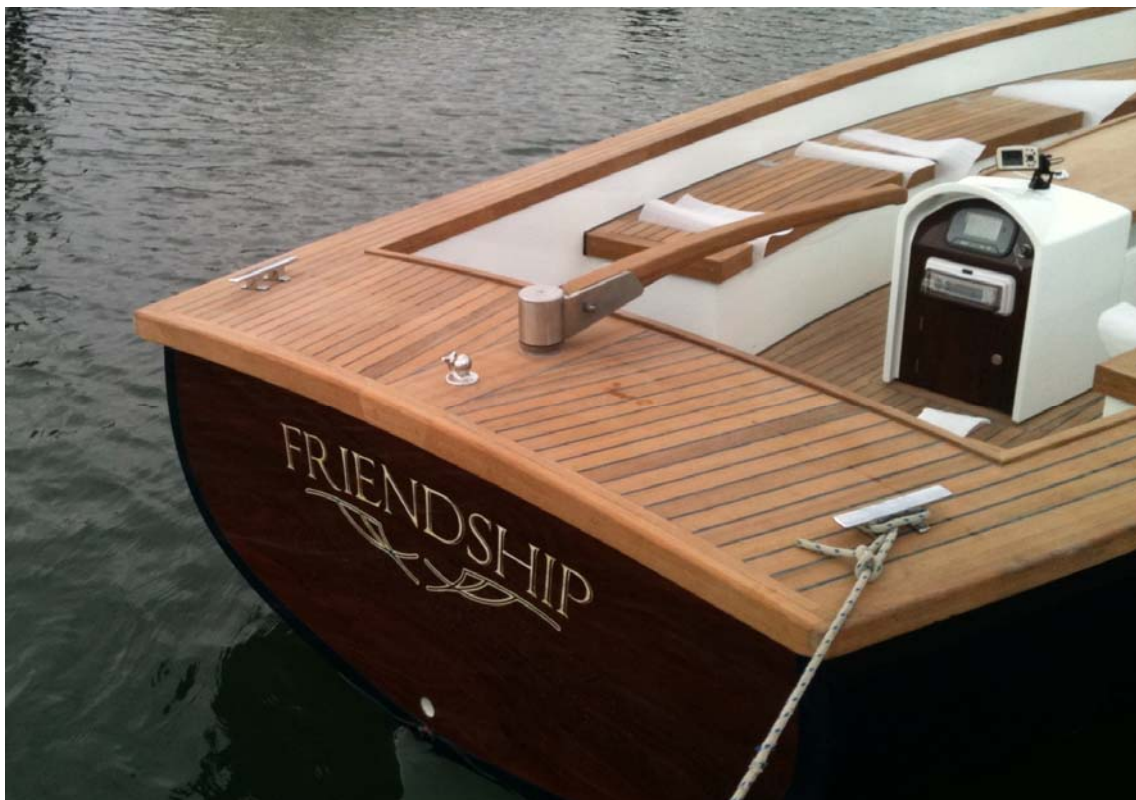
Steering console with graphic display informs on battery charge status, remaining running time, rpm and power consumption
