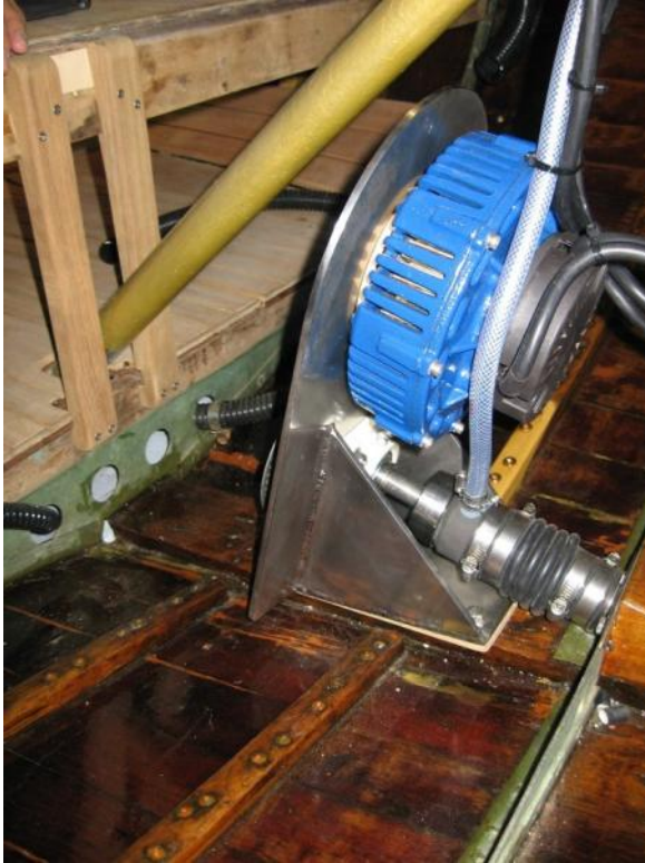
48V DC electric inboard motor
